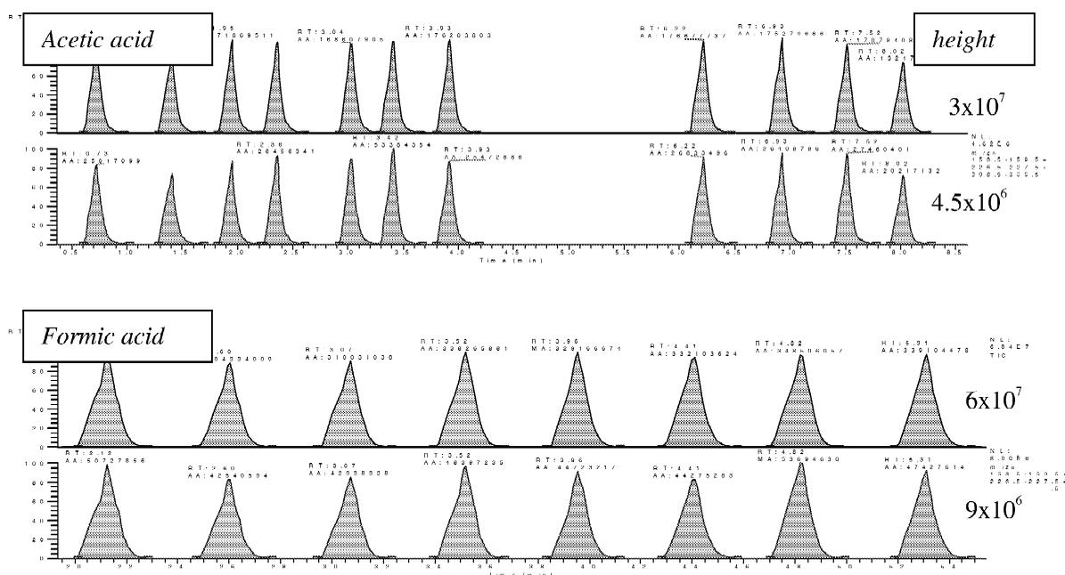
Fig. 2. Comparison of the height of the flow injections for formic acid and acetic acid (the first mass trace is the total ion current, the second mass trace is the sum of the diagnostic ions).
